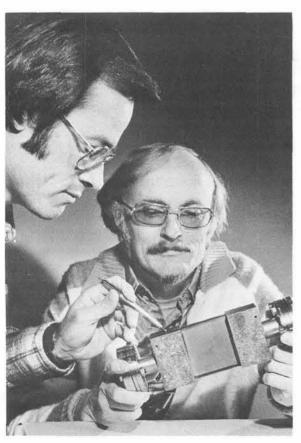
DON COWGILL & FRANK BACON, both of Applied Technology Division 2352, examine target element of neutron generator designed for application to cancerous tissue. Some cancers appear to respond better to neutron treatment than to irradiation with conventional gamma or x-rays.
